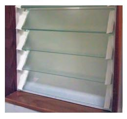
ur vinyl extrusions are made with 100% virgin vinyl materials here in the USA to ensure quality and performance in the Tradewind window. Our fusion-welded 45 degree mitered corners provides for a durable, strong surround frame with a sleek profile that performs as good as it looks. Our louver jalousie windows are weather-tight with concealed corrosion resistant operating hardware. This is not your old school louver jalousie windows from the 1960s.
