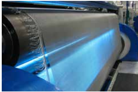
Stainless steel mesh is cut, pre-treated, and powder coated
